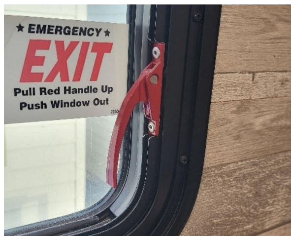
Figure 24. Pull-Lever style latch on an emergency exit. Pull the leverl out, away from base, to disengage latch. Push window out.
