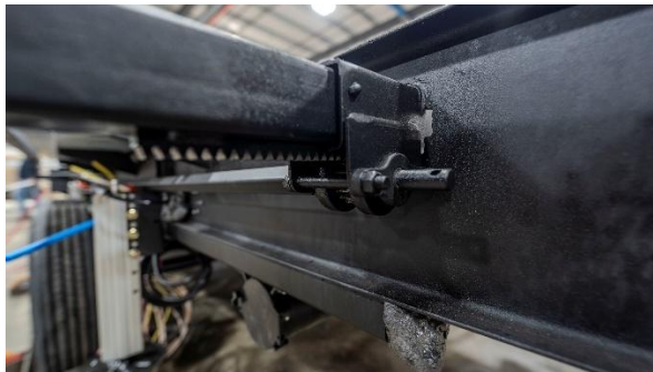
Figure 39. The gear pack is now mounted outside the frame on late-model trailers.
