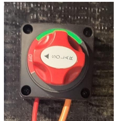
Figure 88. Solar disconnect switch.
