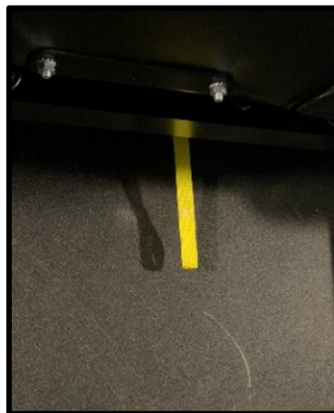
Figure 140. Interior pull strap for opening the ramp door. It is hanging from the top.
