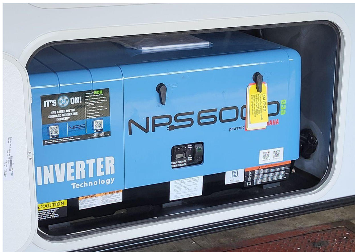
Figure 114. NPS 6000eco generator mounted in the Valor. Note the two black cover removal levers above the NPS logo.
