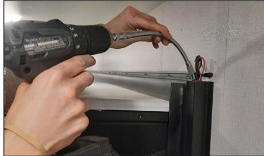
Figure 62. Using the flexible drive tool to manually override the slide.
