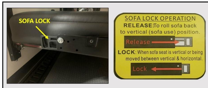
Figure 145. Using the Sofa Lock lever on each side of each sofa base. In the photo, the lever is unlocked (released.)
