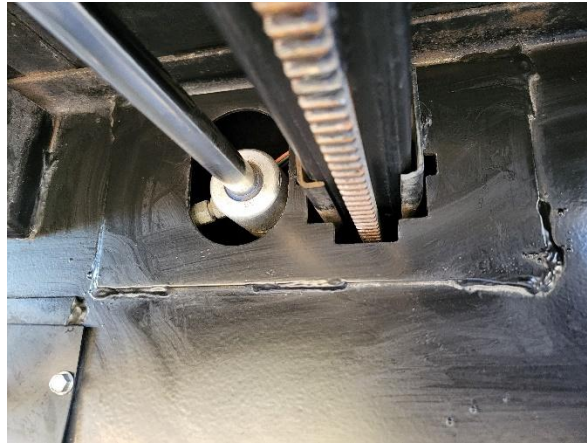
Figure 38. Frame view of the early-model Valor trailers with gear pack inside the frame.
