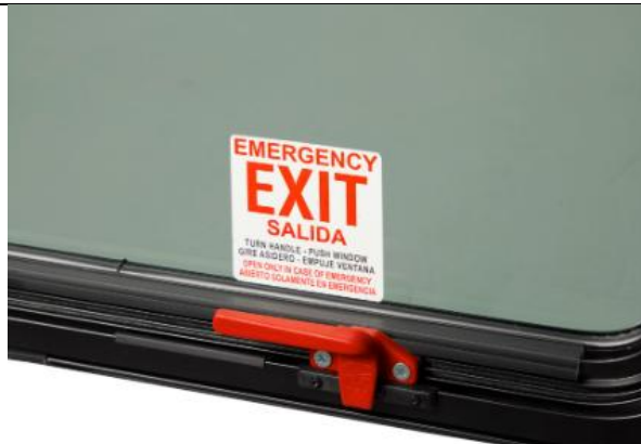
Figure 23. Rotation-Lever style latch on an emergency exit. Rotate the handle up into the window area to disengage the latch. Push window out.
